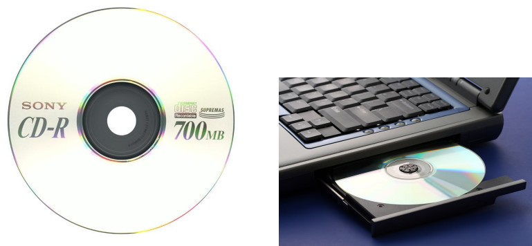
Figura 3.5: Compact Disk i lector de Compact Disks
