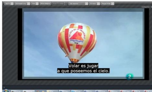
Figure 22. Subtitling application based on web technologies in an HbbTV-compatible PC browser.
