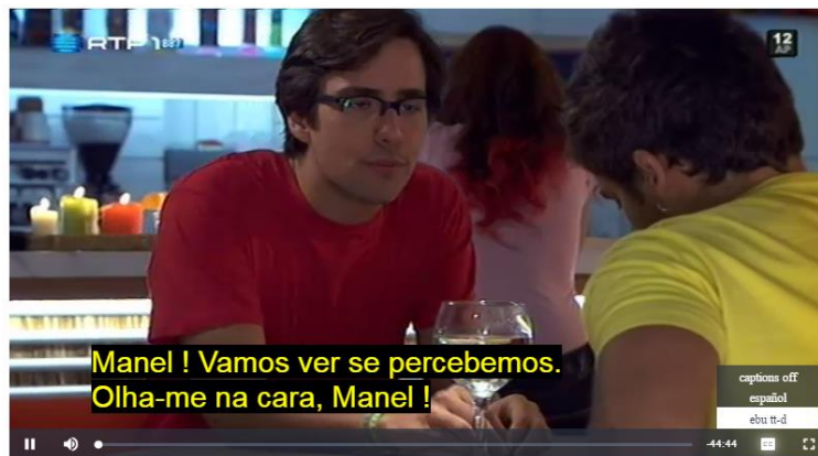
Figure 28. CC button in VideoJS player shows the menu for activating EBU-TT-D subtitles
