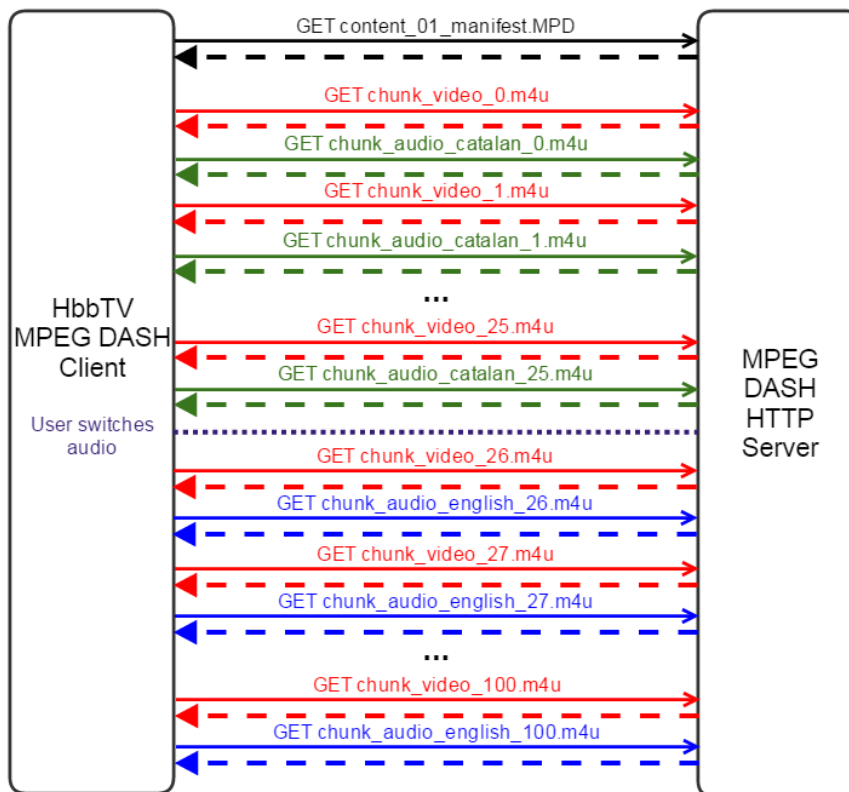
Figure 5. Playback and switching of audio component using MPEG-DASH
