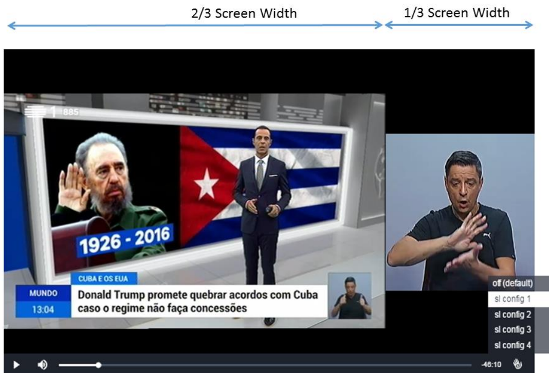
Figure 14. Configuration 1: 2/3 of the screen width is dedicated to the video contents, and 1/3 to sign language video
