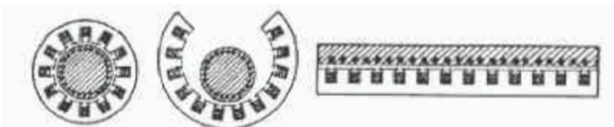
Figure 14. Conversion of a rotating machine to a lineal machine. Source [23]
