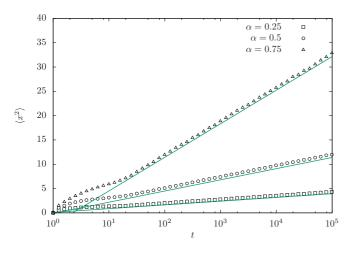
FIG. 1. MSD for the CTRW model with preferential relocation to visited places. Symbols represent the results from Monte Carlo simulations averaged over  $2 \times 10^6$  realizations, while lines correspond to the asymptotic prediction for a Gaussian kernel with  $\sigma^2 = 1$  as in Eq. (17). For the waiting time distribution  $\varphi(t)$  an exponential distribution with  $\tau = 1$  has been used.
