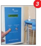
One simple button press starts the chosen sequence of evacuation and replacement of gas in the jar. The same button flashes when the cycle is complete.
