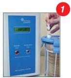
Simply attach the connector from the Whitley Jar Gassing System to the jar containing your samples. Remember to include a catalyst sachet in the jar when preparing anaerobic conditions.
