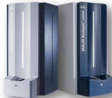
The MALDI Biotyper system is a technique that allows the rapid identification of bacteria, fungi and yeasts through a phenotypic approach based on libraries of microorganisms.
