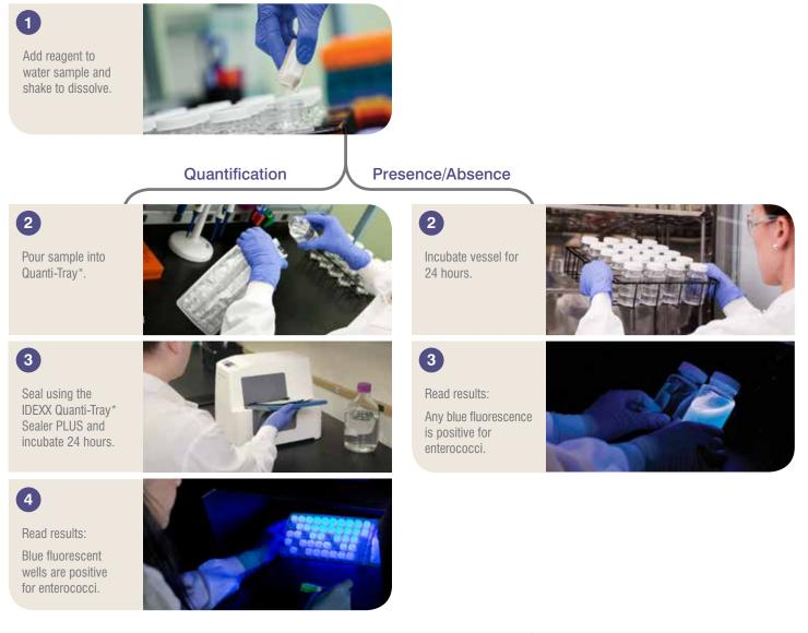
Quanti-Tray\* provides most probable number (MPN) counts of up to 200 per 100 mL sample. Quanti-Tray\*/2000 provides MPN counts of up to 2,419 per 100 mL sample. North/South America: 1-207-556-4496/1-800-321-0207 Europe: 00800 4339 9111 UK: +44 (0) 1638 676800 China: +86 21 61279528 Japan: +81 422 71 5921 Australia: 1300 443 399
