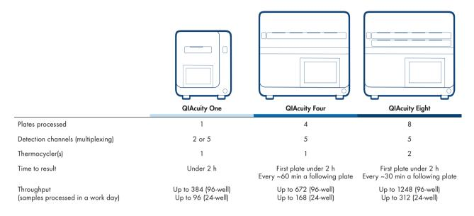
The system offers distinct plate types with partitions designed to accommodate flexible throughput and sensitivity requirements.
