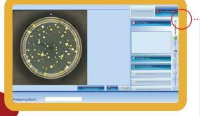
ProtoCOL 3 has two methods of counting: Total Plate Count and Colour Classification. Total plate count gives a quick and accurate count. Colour classification allows colonies to be separated according to colour, size and shape. Colonies grown on membrane filters can also be counted with ProtoCOL 3 using the grid removal function.
