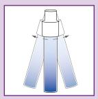
Close the tube with the cap, and shake vigorously by hand for 1 minute to extract the allergen.
