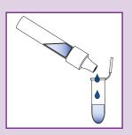
Remove the cap from the extraction tube and replace it with a filtered dropper tip. Transfer the extracted sample to a fresh incubation vial.
