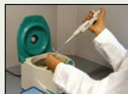
3. Cell lysis / rRNA recovery (2 mL sample, 13'000 rpm, 37°C, 45-60 min)
