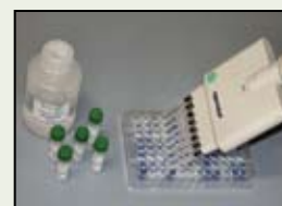
8. Detection reaction (chromogenic Enzyme reaction, 15 min)
