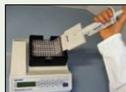
7. Washing (Removal of unbound components, 2 x 1 min)
