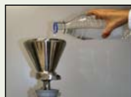
1. Sample filtration (100-1000 mL water, 15 min)
