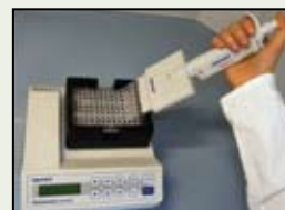
5. Immobilisation (Binding of the "sandwiches" to the binding plates)
