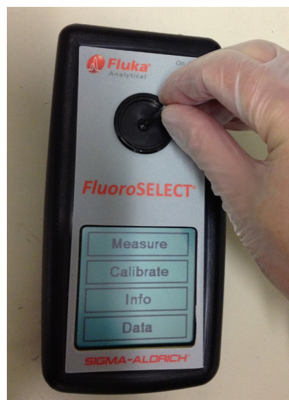
Figure 4: High technology fluorometer with stable high performance LED source and touchscreen.
