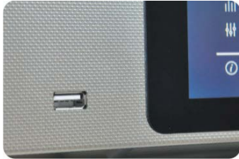
USB port for data download to USB stick and for uploading programs.
