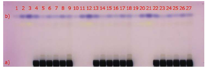
Figure 5. Visualisation of the plate under visible light (white light); a) matrix compounds after staining with anisaldehyde sulphuric acid (black areas); b) 2-methylquinoxaline (blue spot at hRf 80), (reaction product of methylglyoxal with 1,2-phenylenediamine)
