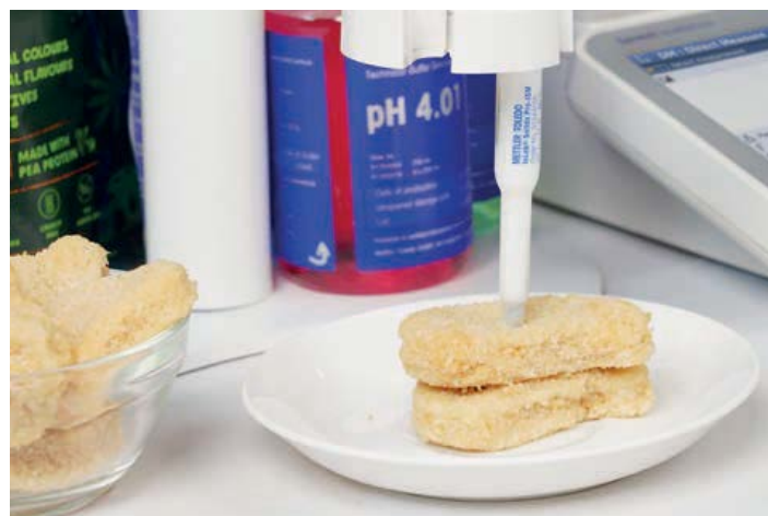
Figure 3. pH measurement of plant-based chicken nuggets using InLab Solids Pro-ISM sensor and SevenExcellence S400 meter.
