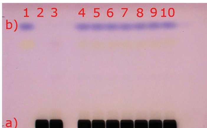
Figure 3. Visualization of the plate under visible light (white light); a) matrix compounds after staining with anisaldehyde sulfuric acid (black areas); b) 2-Methylquinoxaline (blue spot at Rf 80), (reaction product of Methylglyoxal with 1,2-phenylenediamine)
