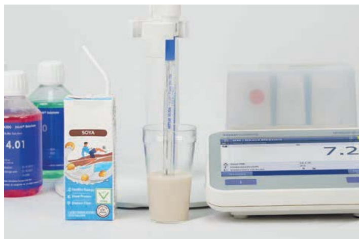
Figure 2. pH measurement of soy milk using InLab Power Pro-ISM sensor and SevenExcellence S400 meter.
