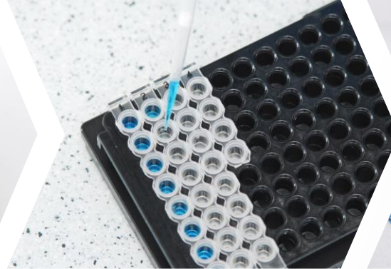
Using stepper pipette, add 10 \mu L of Proteinase K Reagent to Lysis Tubes
