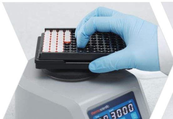
Remove PCR tubes, seal and vortex for 10 seconds and flick to remove droplets
