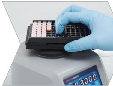
Remove PCR tubes, seal and vortex for 10 seconds and flick to remove droplets
